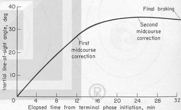
FIGURE 28-2.—Gemini 130° transfer trajectory.
