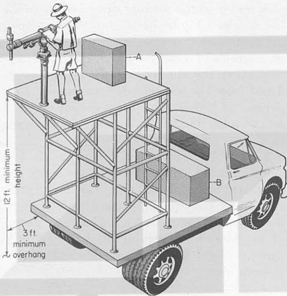
FIGURE 34-23.—Ground-site photoelectric photometer mounted on a truck.
