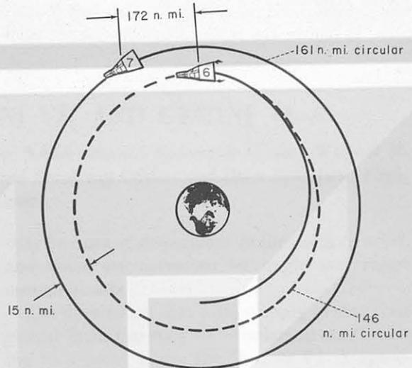
FIGURE 28-8.—Gemini VI-A coelliptical maneuver at third apogee.
