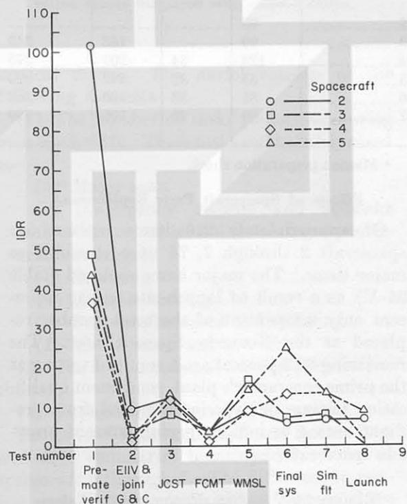
FIGURE 24-2.—Occurrence of interim discrepancy records for individual tests.
