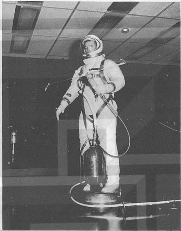
FIGURE 22-14.—Three-degree-of-freedom air-bearing simulator.
