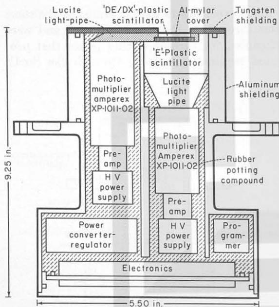
FIGURE 37-3.—Proton/electron spectrometer used for Gemini VII mission.
