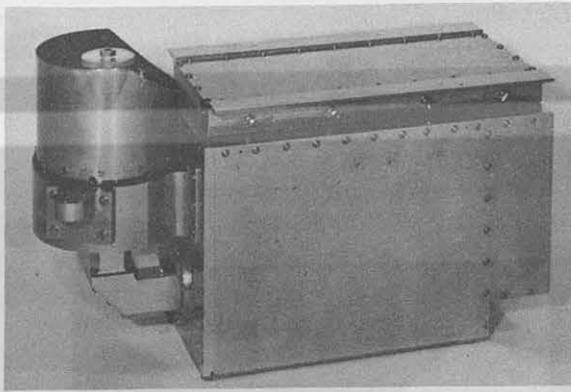
FIGURE 38-4.—Dual-channel interferometer spectrometer.
