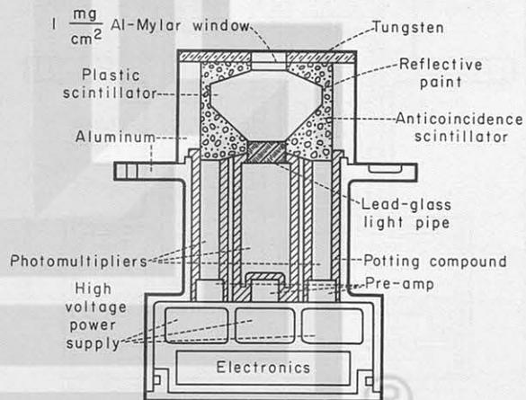
FIGURE 37-1.—Proton/electron spectrometer used for Gemini IV mission.
