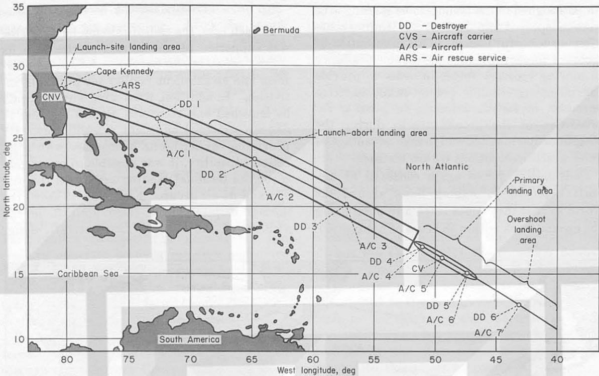
FIGURE 21-9.—Gemini II recovery-force deployment.
