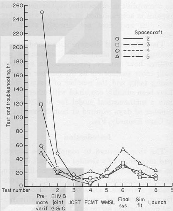
FIGURE 24-1.—Test and troubleshooting time for individual tests.
