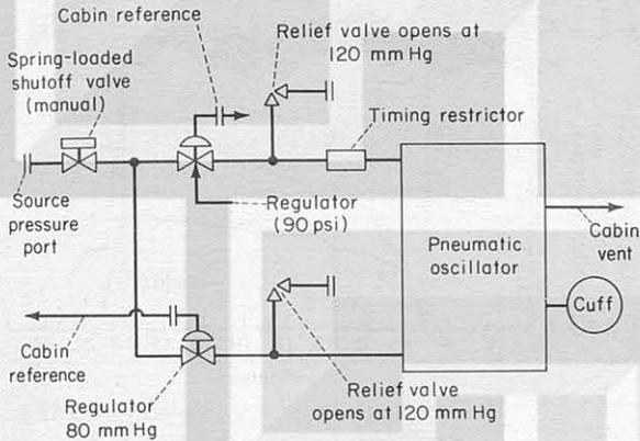
FIGURE 39-7.—Schematic diagram of cardiovascular reflex conditioner.
