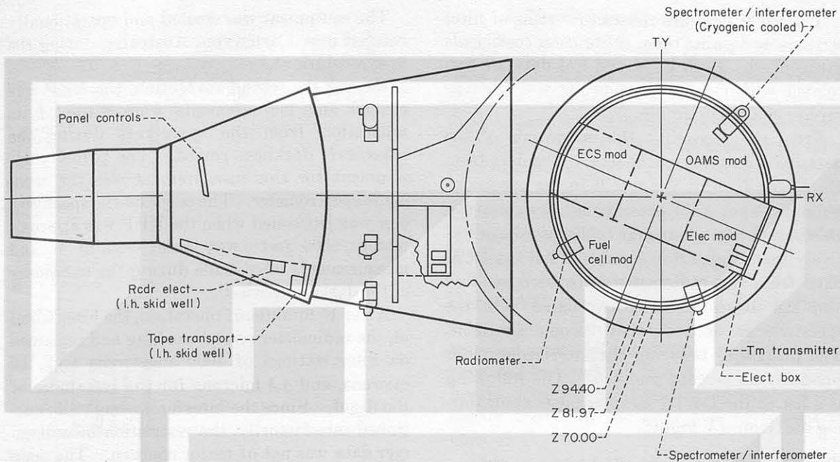
FIGURE 38-10.—Location of Experiment D4/D7 equipment in spacecraft.
