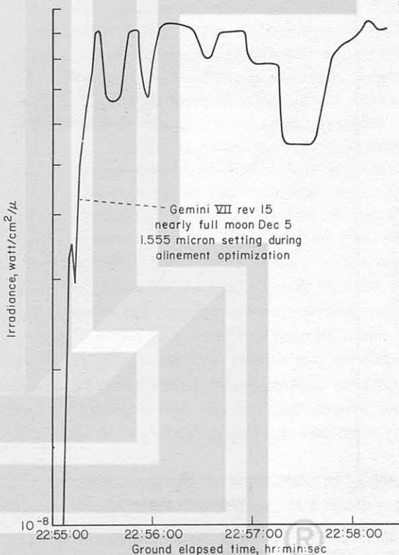
FIGURE 37-17.—Moon irradiance during alinement optimization (1.555 micron setting).
