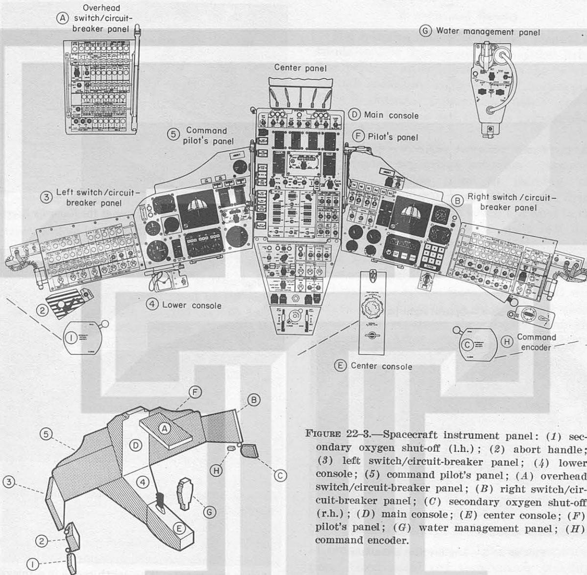
FIGURE 22-3.—Spacecraft instrument panel: (1) secondary oxygen shut-off (l.h.); (2) abort handle; (3) left switch/circuit-breaker panel; (4) lower console; (5) command pilot's panel; (A) overhead switch/circuit-breaker panel; (B) right switch/circuit-breaker panel; (C) secondary oxygen shut-off (r.h.); (D) main console; (E) center console; (F) pilot's panel; (G) water management panel; (H) command encoder.
