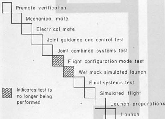
FIGURE 23-2.—Spacecraft test operations performed at launch complex.
