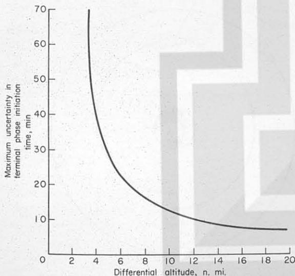
FIGURE 28-3.—Terminal phase maneuver time dispersion analysis.
