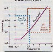
This chart shows the measurement ranges of QSAM. The "Experiment" line represents the level of acceleration a typical Spacelab fluid physics experiment will tolerate.
