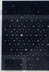
The atomic structure of a quasicrystal is revealed by X-ray diffraction, showing the five-fold symmetry not
