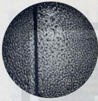
This visual image shows vapor droplets 2 hours after the onset of phase separation. The domains are not uniform because of the laser beam that was present at the beginning of the experiment. Its influence is still not understood and will be investigated during Dr. Beysens' experiment.
