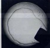
This visual image of SF<sub>8</sub> shows two phases at T = T<sub>C</sub> - 3 mK. The most notable feature is the variable and small surface tension around the large central vapor bubble. This vanishing surface tension is a trait of fluids at their critical point. Similar phenomena will be investigated during Dr. Ferrell's experiment. The bar at the right bottom is the stirrer. (No stirrer will be used on IML-2.)
