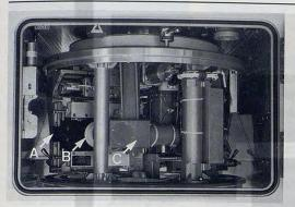
The NIZEMI facility centrifuge (A) Sample Holder; (B) Microscope Objective; (C) Video Equipment
