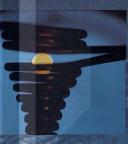
A. Metals and alloys can be positioned using electromagnetic forces and can be processed without containers, which sometimes contaminate samples. This processing technique cannot be used on Earth as effectively as in low-gravity orbit.
