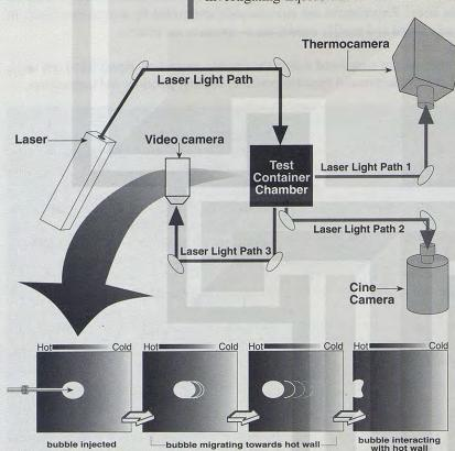
bubble growth, evaporation, and condensation. Such phenomena are difficult to observe on Earth because their effects are masked by gravity-induced fluid movements. Knowledge gained through the use of the BDPU will test and refine theories of fluid behavior, and may be used to improve the design of spacecraft life support and fuel management systems, as well as materials processing both on Earth and in space.
