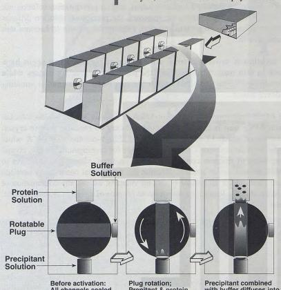
Before activation: All channels sealed, plug contains buffer solution
