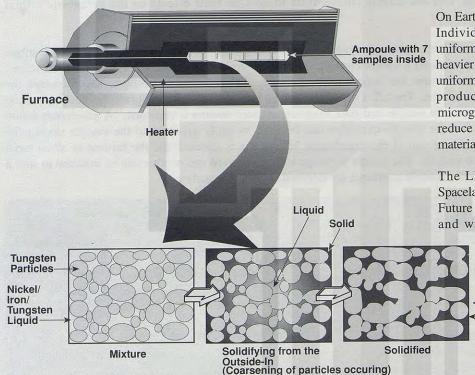
On Earth, gravity can affect the processing of materials. Individual components of a material may not be uniformly mixed because of sedimentation (settling of heavier components from lighter), resulting in a nonuniform internal structure and composition in the solid product. Experiments have shown that the microgravity environment of Earth orbit can greatly reduce or eliminate some of gravity's effects during materials processing.
