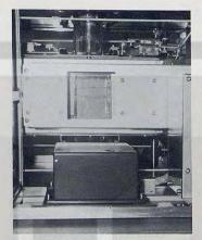
A window in the VIBES unit allows video observation of experiments conducted with and without damping.
