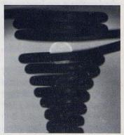
This levitated, molten sample is held within an Earth-bound electromagnetic heating and positioning coil system, which is similar to the one used by TEMPUS. In 1-g, the electromagnetic force must be very powerful to counteract gravity. This deforms the sample and agitates the melted alloy. In microgravity, these problems should be circumvented, allowing materials to be processed without containers that sometimes contaminate the final product.
