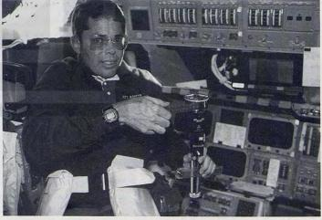
The MAS is used to collect microbes inside the Spacelab.
