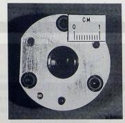
The small center area is the test cell where CPF experiments take place.
