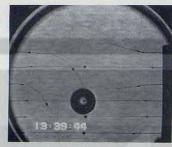
This vapor bubble was generated during the reduced-gravity portion of a KC-135 aircraft's parabolic flight.
