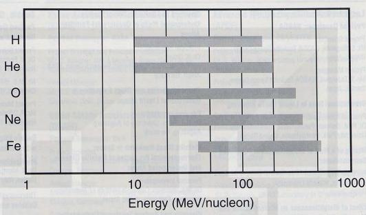
This chart shows incident particles that the RRMD will identify and the energy ranges the device can detect.
