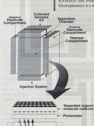
RAMSES separates biological materials on the basis of their electrical charge and polarity.
