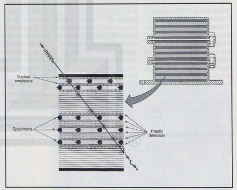
When cosmic particles pass through the Biostack, they deposit their high energies in layers of radiation detectors and live specimens.
