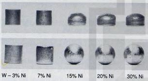
The top row of tungsten (W) - nickel (Ni) samples was sintered at 1450 °C for 60 minutes on Earth; the bottom row was sintered in the LIF at 1450 °C for 60 minutes during the Spacelab-J mission. When the percentage of nickel in the specimen increases, the sample tends to behave like a liquid, resulting in the spherical configuration in space.
