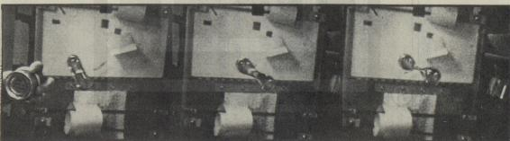
IF A FREE-FLOATING DROP IS ROTATED IN A LOW-9 ENVIRONMENT, SURFACE TENSION FORCES CAN BALANCE CENTRIFUGAL FORCES TO ESTABLISH AN
