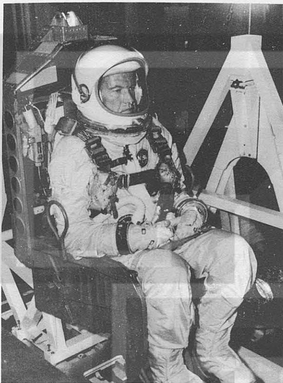
FIGURE 3-14.—Gemini ejection seat.
