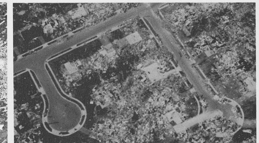
[F5] INCREDIBLE DAMAGE (261 - 318 mph) Strong frame houses lifted off foundations and carried considerable distance to disintegrate; automobile-sized missiles fly through the air in excess of 300 ft; trees debarked; incredible phenomena will occur.
