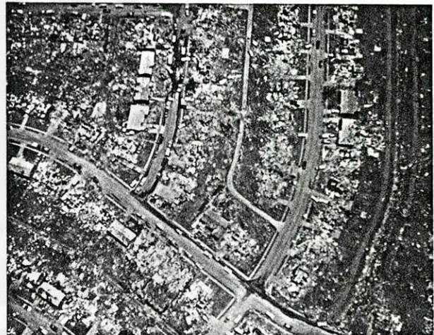
Fig. 10 One, two, and three houses left untouched by the Wichita Falls, KS tornado of 10 April 1979 because they were located between a number of intersecting tracks of suction vortices. Photo by Ted Fujita.
