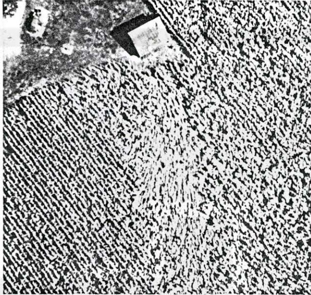
Fig. 27 A microburst airflow deflected by a tin roof during the downburst storm of 30 September 1977. Photo by Ted Fujita at Kingman, IN. From Fujita (1978).
