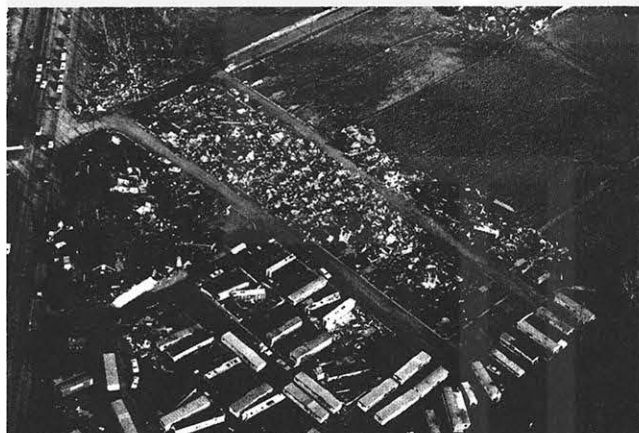
FIGURE 23.—Aerial photograph of severe damage to the Midway Trailer Court northwest of Goshen, Ind. The devastation near the center of the picture was caused by the left funnel of the tornado shown in figure 31. The right funnel moved over the plowed field from right to left, cutting across the upper corner of the court. For more detail see figure 52. Damage occurred at 1732 CST on April 11; the picture was taken on April 13. For exact location refer to figure 22.
